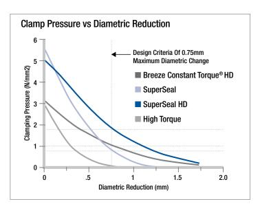
Super-Seal HD w/Belleville washers generates approximately 60% greater clamping pressure than Breeze Constant Torque® HD clamp.
