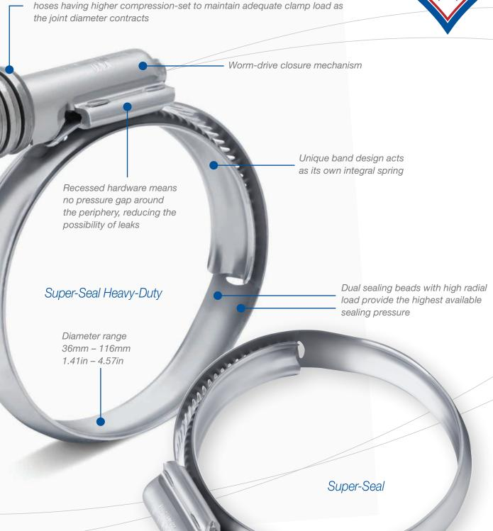
Available with or without Belleville washer springs, which can be used on
