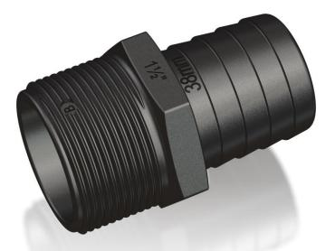
TruDesign Tails are moulded from a glass reinforced nylon composite. High strength, high-modulus glass fibers impregnated into the nylon provides dramatic strength, stiffness, toughness, and dimensional stability. TruDesign Tails eliminate the corrosion and electrical bonding problems associated with metallic fittings. The Tails are designed for twin hose clamps, and do not crush under high load conditions.
