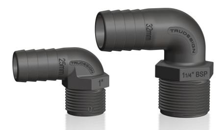
TruDesign Tails are moulded from a glass reinforced nylon composite. High strength, high-modulus glass fibres impregnated into the nylon provides dramatic strength, stiffness, toughness, and dimensional stability. TruDesign Tails eliminate the corrosion and electrical bonding problems associated with metallic fittings. The Tails are designed for twin hose clamps, and to not crush under high load conditions.
