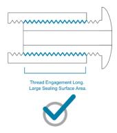
To comply with International Marine Standards, all TRUDESIGN™ Skin Fittings, Ball Valves and threaded connectors are manufactured with parallel threads. This ensures threaded connections utilise full thread engagement, resulting in greater strength and sealing ability. A backing nut can be used to help secure fittings in the desired direction.
