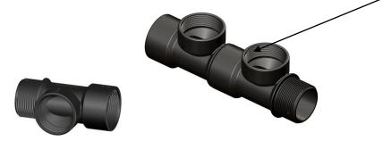
Align the two location notches. There is no need to tighten fully. When adhesive type thread sealant is used, fittings need only be "finger tight" as the sealant will provide full waterproofness and structure once cured. This allows the two fittings to align.
