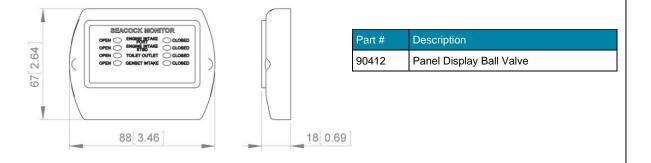
The Position Monitoring function switches state when the Ball Valve is in the open position.
