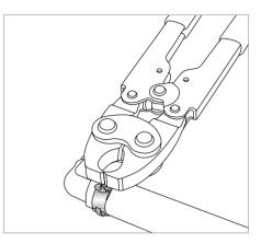
3. Cut through the ear and remove the clamp carefully.
