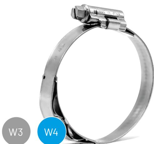
12mm bandwidth Constant Tension worm-drive clips are designed to be used primarily in the automotive sector. The main advantage of this clip over the standard Mikalor worm drive is to be found in the spring-loaded insert, fitted on a semi-circular support to the inside of the band.
