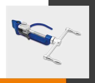
The Loob screw banding tool is used to tension stainless steel bands with width of up to 20 mm in all steel grades offered by Loob. It is made of corrosion-resistant galvanized steel. The tool also has built-in blades for cutting through stainless steel. It is used together with banding buckles. The banding machine is suitable for use in a variety of environments.
