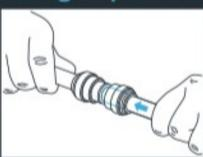
Push the pipe up to the pipe stop.
