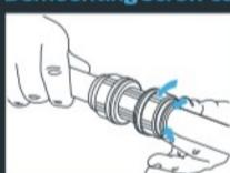
To disconnect, ¼ turn the screw cap, push the collet and remove the pipe. Fittings are reusable.
