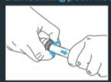
To disconnect, ensure the system is depressurised. Push the collet towards the fitting and remove the pipe. Fittings are reusable.
