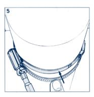
Hold down any excess band just before the buckle is clamped. Finally tighten with the ratchet spanner.
