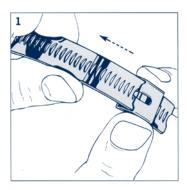
Slide the buckle onto the band in the direction of the arrow and push around to the housing.
