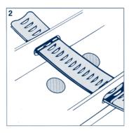
Thread the band through the slots in the sign and around post.
