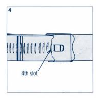
Locate the tongue of the buckle in the 4th slot of the band. Screw the band through using a hand or power tool.
