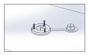
9. Use a screwdriver or drill to drive the three screws into the adapter ring from the top side.
