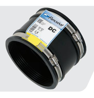
Flexseal Drain Couplings are used to connect, repair and maintain drainage systems and other small diameter non-pressure pipelines. Available to suit any pipe material up to 275mm outside diameter, Drain Couplings are designed for use in drainage systems where the resistance to earth loads (usually provided by a Standard Coupling) is not required.
